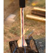
The original back panel for the signal cannot be used so cover the back with black plastic insulating tape.as shown here.
